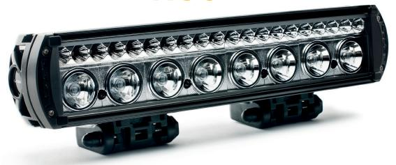
A world first when introduced and still setting the standard, the RS-8 features three ECE approved functions in one compact unit. During daytime driving, the 20 x 0.5W LEDs illuminate to become daytime running lights (DRL). When the vehicle side lights are switched on by the driver, these LEDs run at reduced intensity, while switching on the vehicle High Beam, activates the 8 x 11W LEDs, to deliver exceptional visibility through to 350m+.
